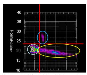
The RadEye SPRD-GN's CLYC and PSD filters provide clear delineation between the gamma radiation of interest (light blue), high energy charged particles typically from cosmic rays (yellow), and neutrons (blue).
