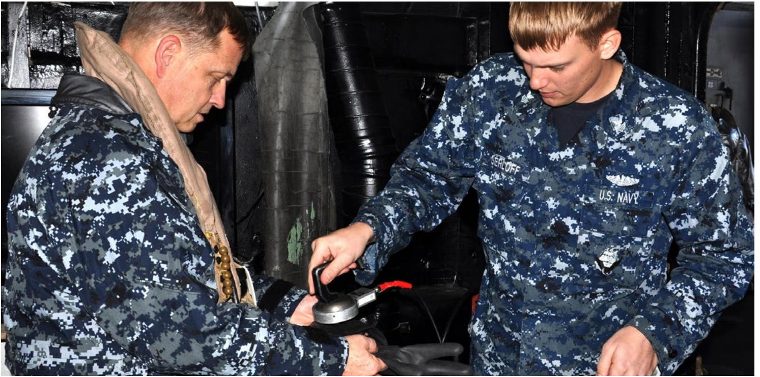
A petty officer assigned to the USS Frank Cable, a submarine tender, uses a RADIAC meter on another officer to monitor possible radiological contamination. (US Navy photo by Petty Officer 1st Class Kim McLendon.)
