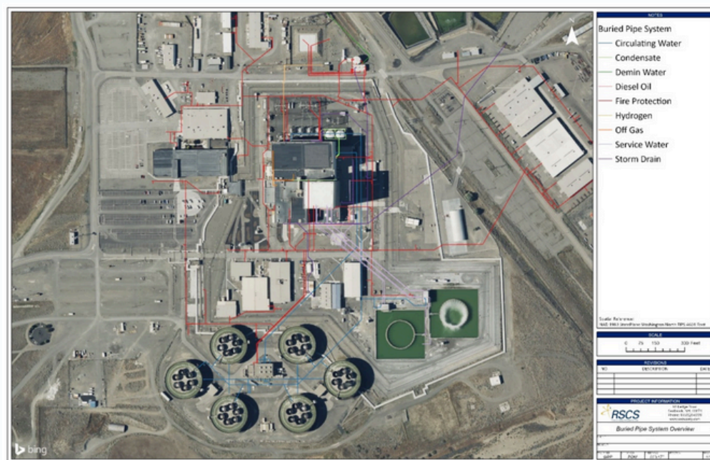
GIS depiction of a nuclear facility buried piping digital twin (pipe centerlines and systems shown)
